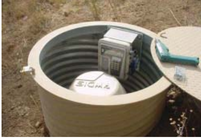
Typical automated flowmeter, sampler and housing used in Lake Tahoe.
